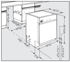
1) with 35" (890 mm) machine height 2) with 33 1/8" (840 mm) machine height Range of adjustment is approximately 2" (5 cm).
